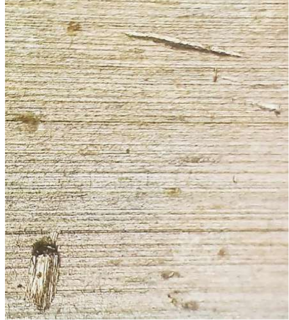
Metallic particles inclusion (40X). Unacceptable
