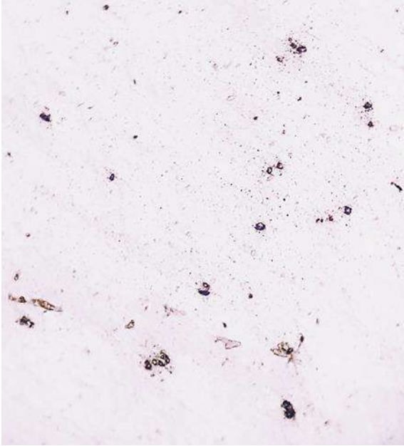
Pick-up (comet tail appearance). Unacceptable
