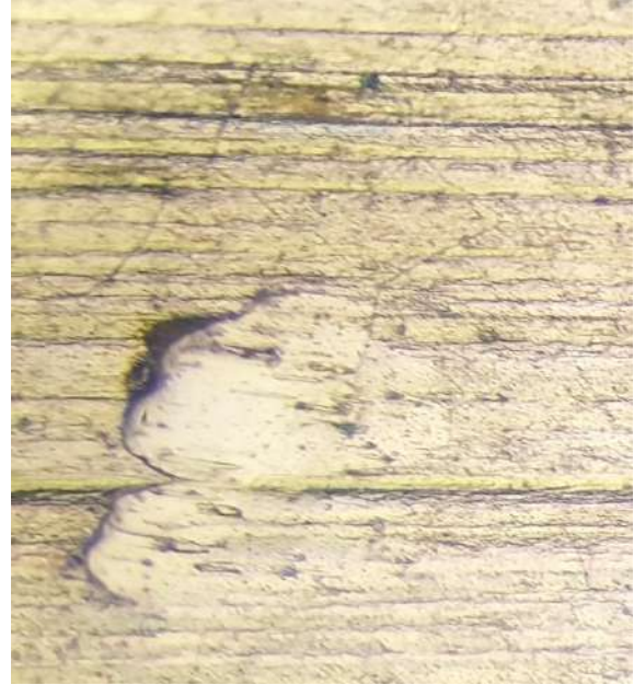
Metallic particles inclusion (40X). Unacceptable
